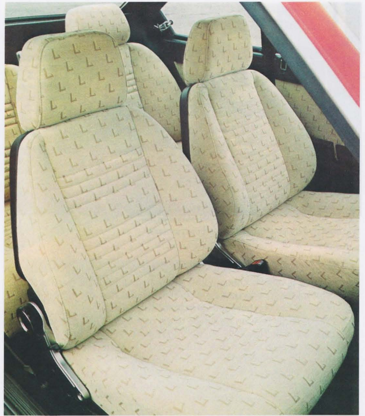
German market Series two coupé seats. Superb 'L' cloth (also used in the Gamma) was specially commissioned by Lancia from luxury tailors and clothmakers Ermengildo Zegna best known for their 'yachting' range of clothing. Cloth was more expensive to replace than leather.
